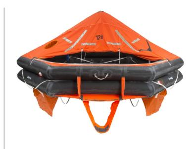
Upon release from its stowage arrangement, this type of liferaft either slides automatically or is thrown overboard manually. Once waterborne, the liferaft inflates by a firm pull to the painter line.
